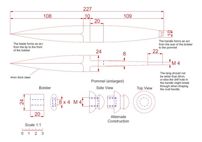
BLADE Use any accepted blade steel, 4mm thick.
